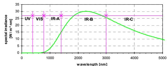
The simulation shows that the major output of radiant exitance power is in the IR-B (56.87 %) and the IR-C (37.95 %) region of the irradiated spectrum, with a total radiant emittance power of 9356 W (Stefan – Boltzmann law).
