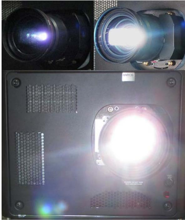
Fig. 2. As example, a >10 000 lm projector, for the photo on the left switched to black state, while for the photo on the right the image is full white, both viewed from outside of the beam. The lower photo shows intra beam viewing during the black state.
